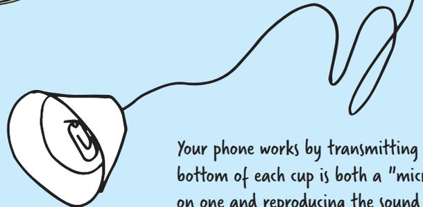
Your phone works by transmitting sound vibrations along a tightly-pulled string. The bottom of each cup is both a "microphone" and "speaker," picking up sound vibrations on one and reproducing the sound at the other.
